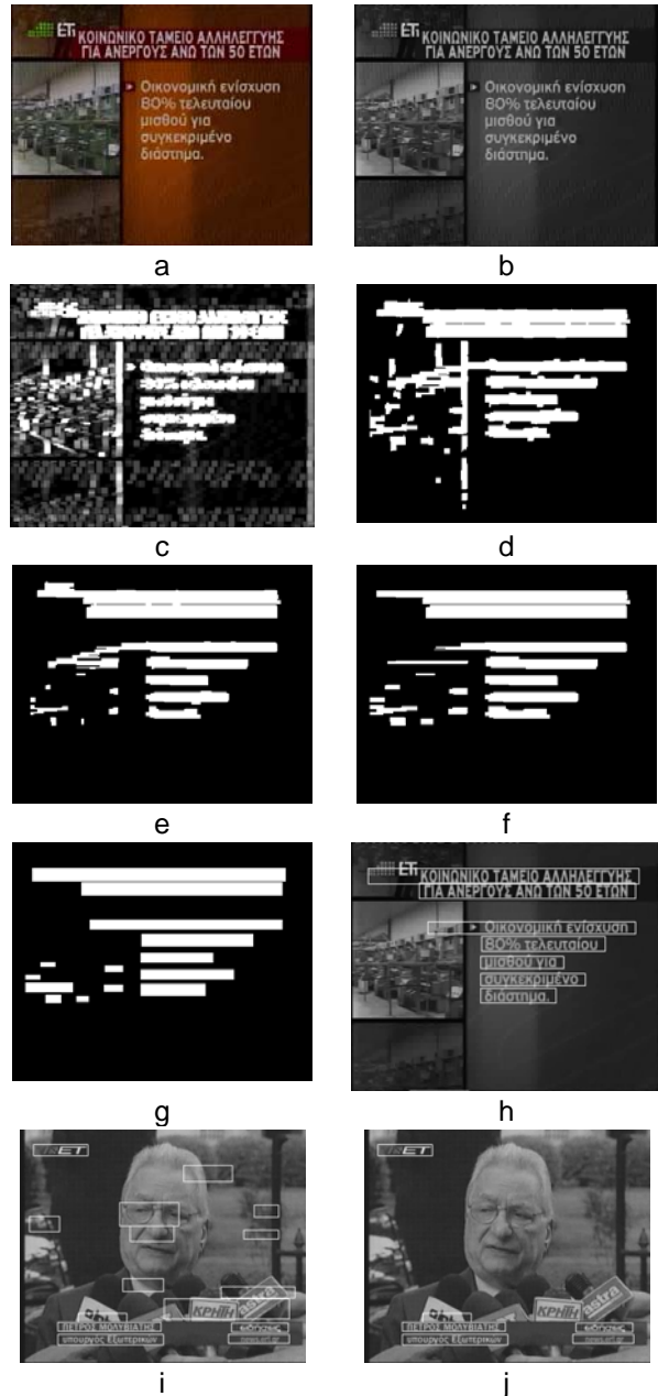
Figure 2. The intermediate results of the text localization process: (a) original, (b) gray scale, (c) filtered, (d-g) , (i-j)
